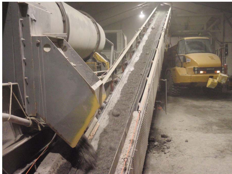
Photo 11: View of FCM exiting the chute at the FCP. Note that at the time this picture was taken a higher frequency of frozen clumps were being noted in the FCM. Shortly after this picture the FCP was temporary stopped while an overloaded belt, from the hopper, was fixed.
